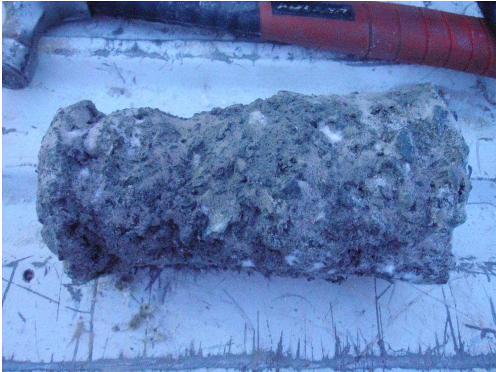
Photo 10: ~ HB12-ND-DC14-20120201, taken from 1+60 centerline. Note the very poor quality of the core. Material was taken just after lift reached -2°C (according to the installed single bead). As the lift was just frozen the core melted/ outside did not core nicely due to the higher temperatures.
