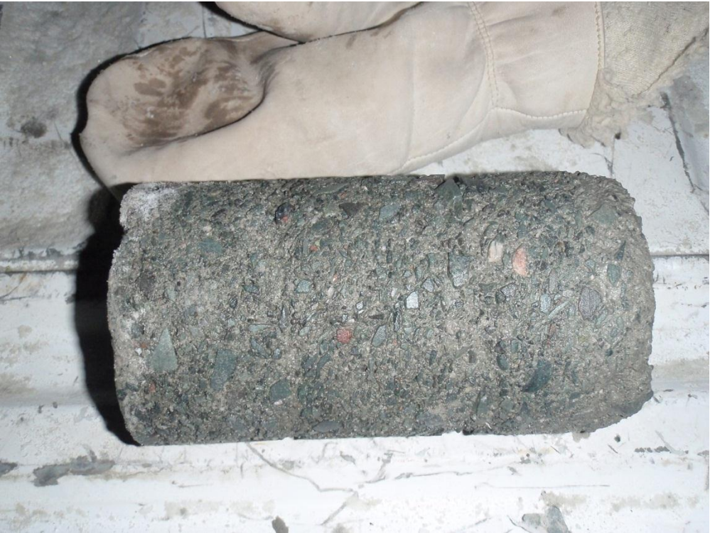
Photo 11: HB12-ND-CORE-DC15-QA-20120201 taken from ~ 1+75 on the downstream. Note that this lift had been frozen for a few days now.
